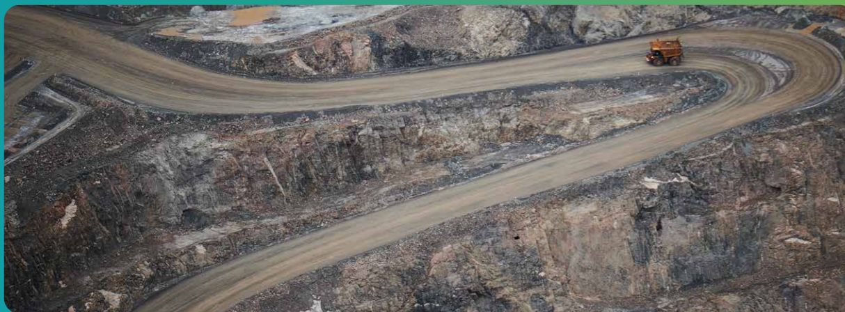
Water cart conducting dust suppression activities at KCGM, Kalgoorlie Production Centre, Western Australia
